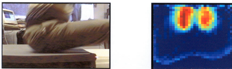
Figure 7: Video frame and pressure image of stumble event
