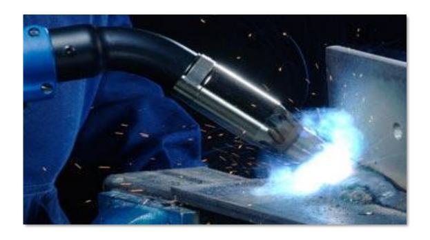
The extraction system is attached directly to the tool and draws the contaminant though the tool directly at the source.
